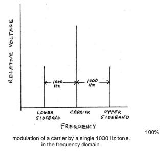
The two sidebands are a result of how the AF and RF sine waves are mixed in the transmitter - they are multiplied. When two sinusoidal waves are multiplied and the DC offset is positive, trigonometry tell us that:
