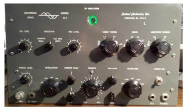
This is a wonderful, well designed 20-Watt vacuum tube single sideband exciter with full HF band coverage for that era, upper and lower sideband modulation, AM, PM, CW, and voice operated relay (VOX)
